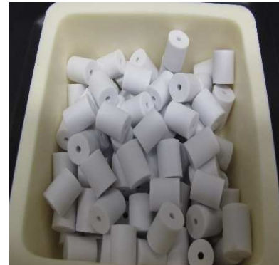
Figure 5 Sintered Al_2O_3 pellets with hole
