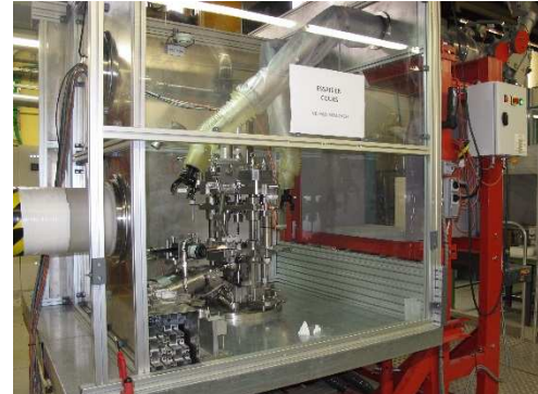
Figure 3 Press in mock-up for remote handling trials
