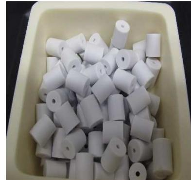
Figure 5 Sintered  $Al_2O_3$  pellets with hole
