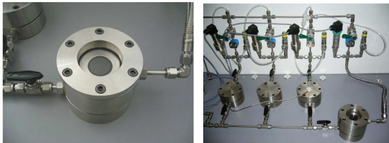
Permeation cell and test bench
