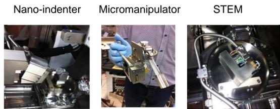
The FIB SEM is a Carl Zeiss Auriga 40 equipped with an Orsay Physics COBRA FIB column. The nano-indenter and the micro-manipulator are mounted on the door of the SEM chamber and the STEM is installed on the stage. All these accessories have to be positioned and connected manually via the gloves, prior to the loading of the radioactive samples. The EDX and the STEM detector must only be used on micro-samples with very low irradiation levels to avoid damage to the sensitive parts of the detectors.
