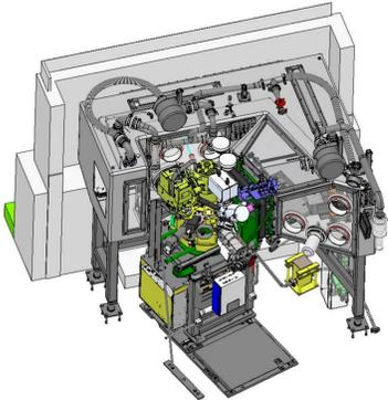
A new **FIB SEM** is operational for **research on nuclear fuels** at the CEA Cadarache. The microscope is installed in a shielded room. It is connected to a glove box, containing the contamination of the samples. The loading of the samples on the FIB SEM stage is done using bar manipulators.
