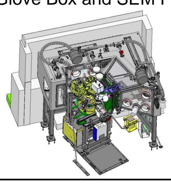
A **new FIB SEM** is operationnal for research on nuclear fuels at the CEA Cadarache. The microscope is installed in a shielded room. It is connected to a glove box, containing the contamination of the samples. The loading of the samples on the FIB SEM stage is done
