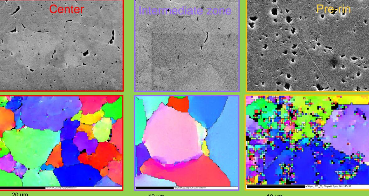
An irradiated UO2 fuel was analysed by EBSD to observe the grains. Different radial positions in the fuel were studied: here, the center, the intermediate zone, the pre-rim and rim. The grain boundaries have been drawn for a misorientation superior to 10°. In the rim, the initial grains are subdivised in smaller grains.
