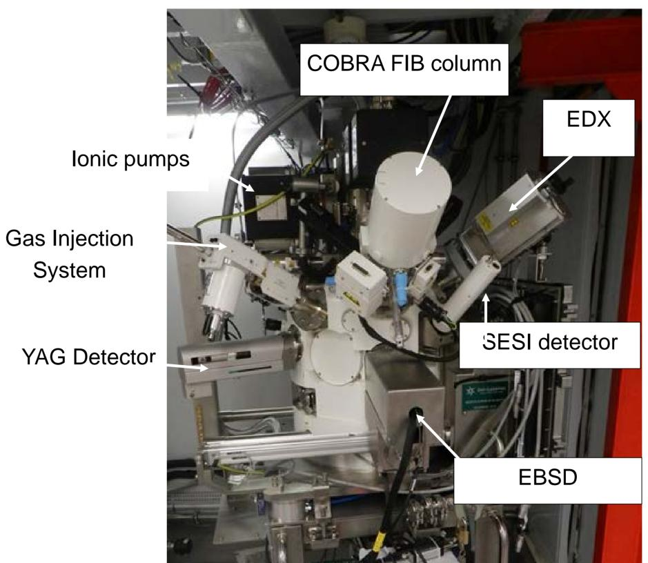
The FIB SEM is a Carl Zeiss Auriga 40 equiped with an Orsay Physics COBRA FIB column.
