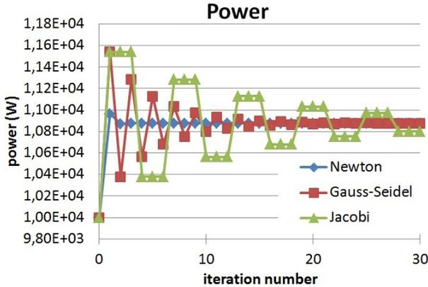
Fig. 2. Global power from different coupling techniques.
