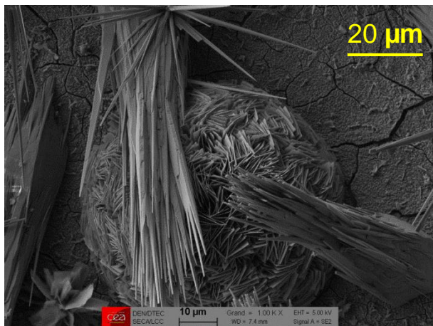
UO 2 pellet lixiviated with iron
