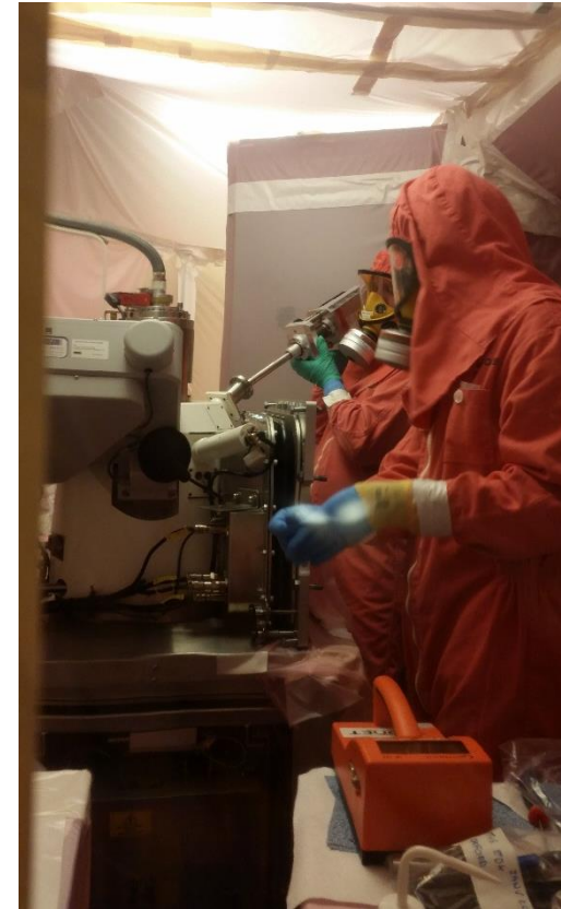
EDS chip replacement
