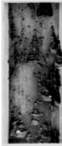
Corrosion of pipes in SCCO 2 storage system from G. Schmitt, White paper, WCO, 2009
