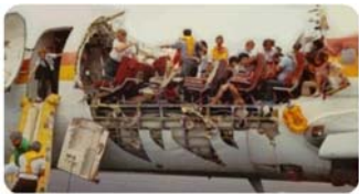
Corrosion cracking of the fuselage of airplane (April 28, 1988 – 1 fatal over 95)
