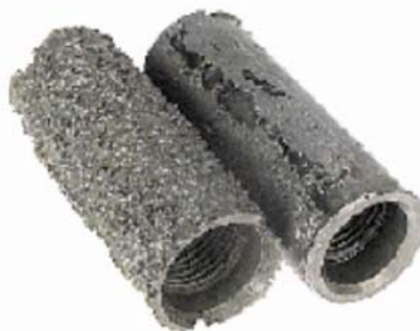
Corrosion of pipes in SCCO 2 storage system from G. Schmitt, White paper, WCO, 2009
