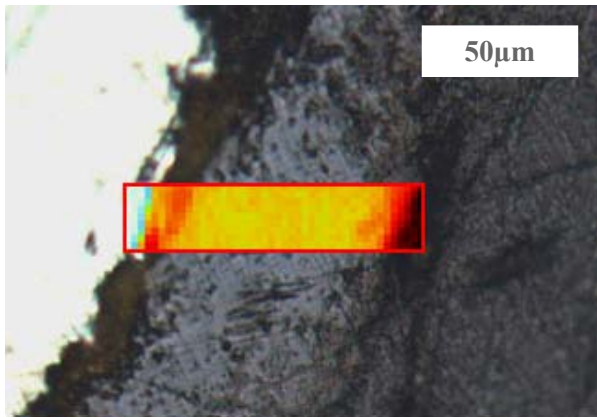
Isolating layer (goethite): reaction at the interface metal/oxide
