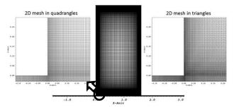
Fig. 6: Basic 2D meshes on rectangles and triangles.
