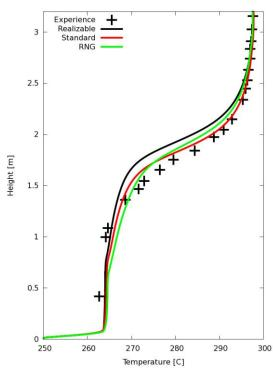
Fig.9: Comparison of measurement and calculation at x=0.1m (FLUENT)
