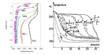
Fig. 4: Transient experiment; variation of vertical temperature profiles with time (left) and local temperature course at selected heights in the cavity (from ref.(3)).
