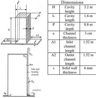
Fig. 2: SUPERCAVNA test section and geometry.
