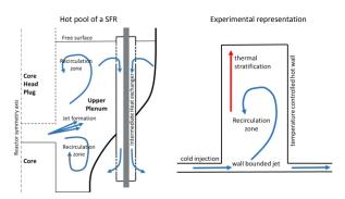
Fig. 1: Flow in the hot pool of a SFR (left) and its simplified experimental representation (right).
