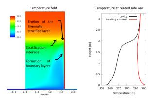
Fig. 7: Temperature distribution in the cavity and the sidewall heating channel.
