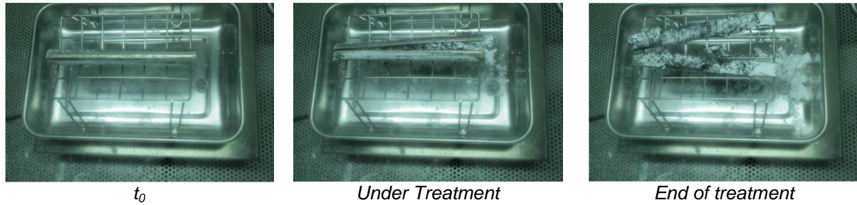
FIG. 3. Illustration of the carbonation treatment of sodium contained into a mock-up of absorber pins
