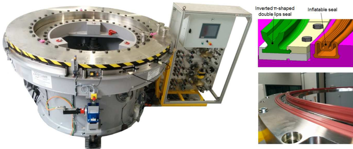
FIG. 4. Left : The Rotary Plug Test-stand. Right: The two seals proposed mounted in their groove
