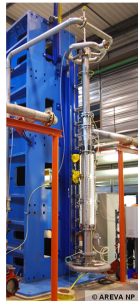
Fig. 12: Test loop for dashpot hydraulic test – AREVA NP Technical Center
