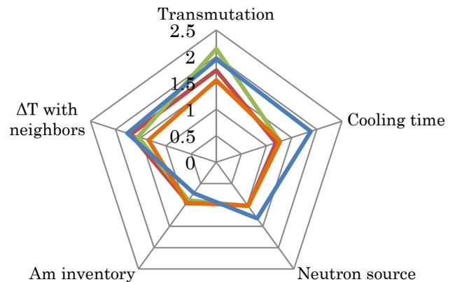
**Figure 7 : Radar plot showing the various impacts of the fissile material studied here. The red curve corresponds to <sup>235</sup>U, the green one to Pu<sup>239</sup>, the orange one to Pu 2035 and the blue one to the moderated case using ZrH<sub>2</sub>.**
