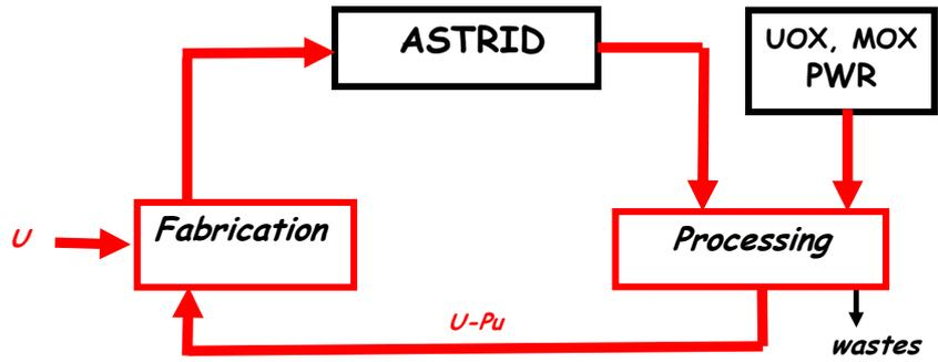
Figure 1: closed fuel cycle for ASTRID
