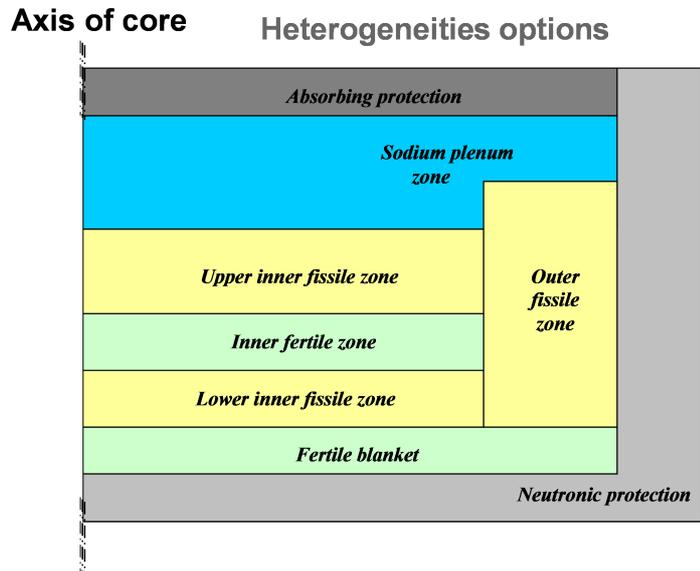
Figure 2: RZ cut of the CFV core
