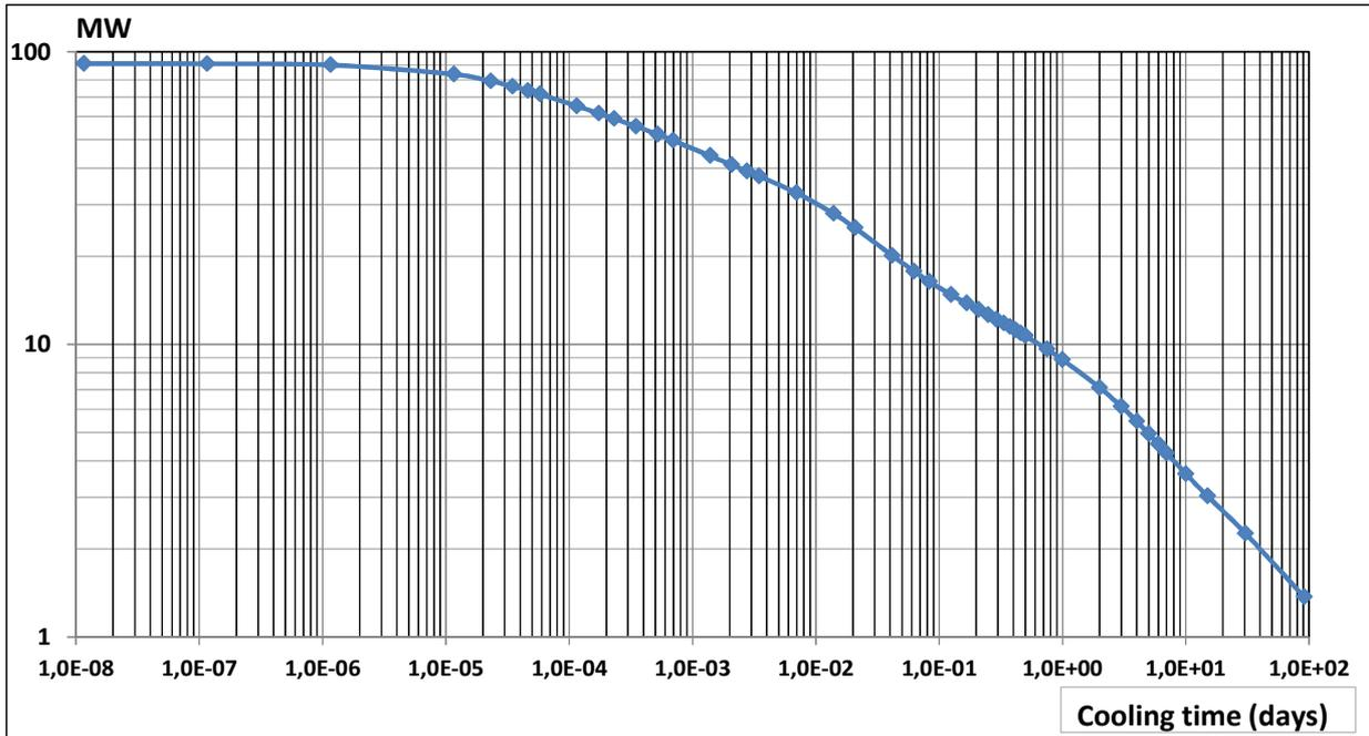
**Figure 7: Decay heat of the “CFV BD 16/10” core**
