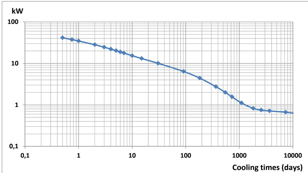
**Figure 9: Decay heat of the spent S/As fuel “CFV BD 16/10”**
