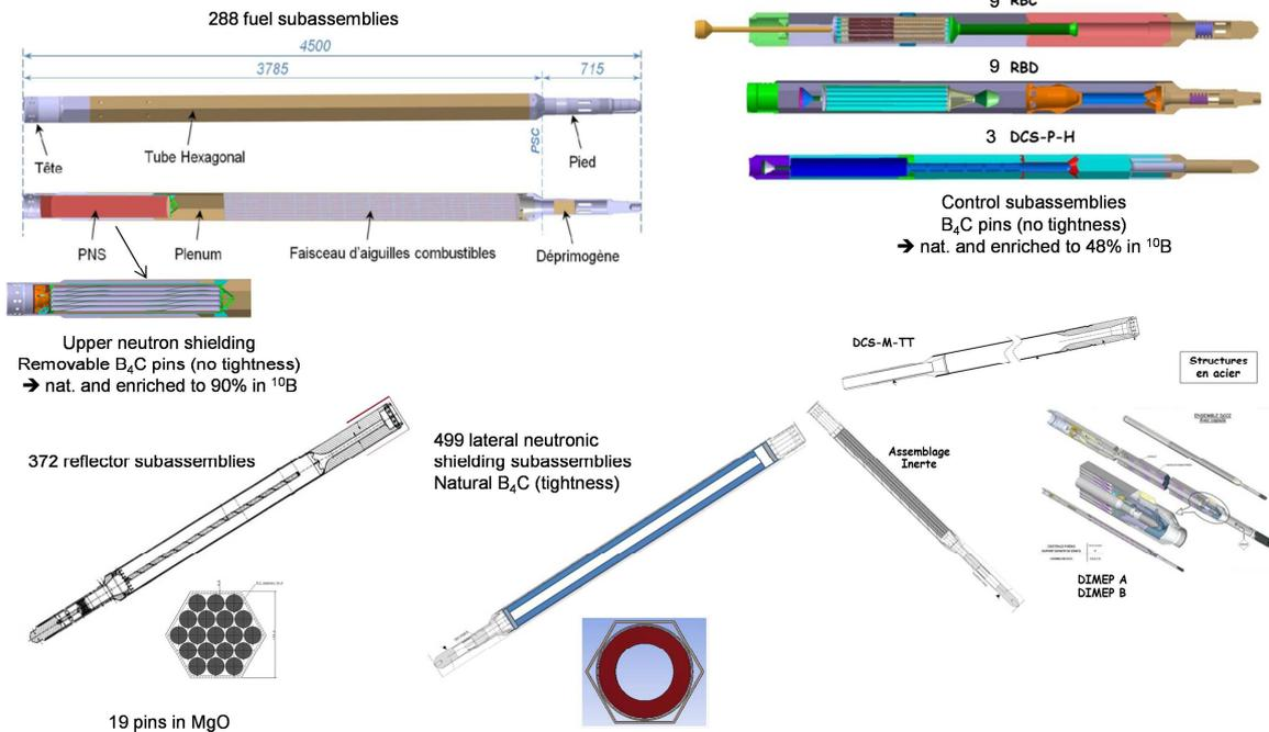
**Figure 5: Different types of subassemblies in the core**
