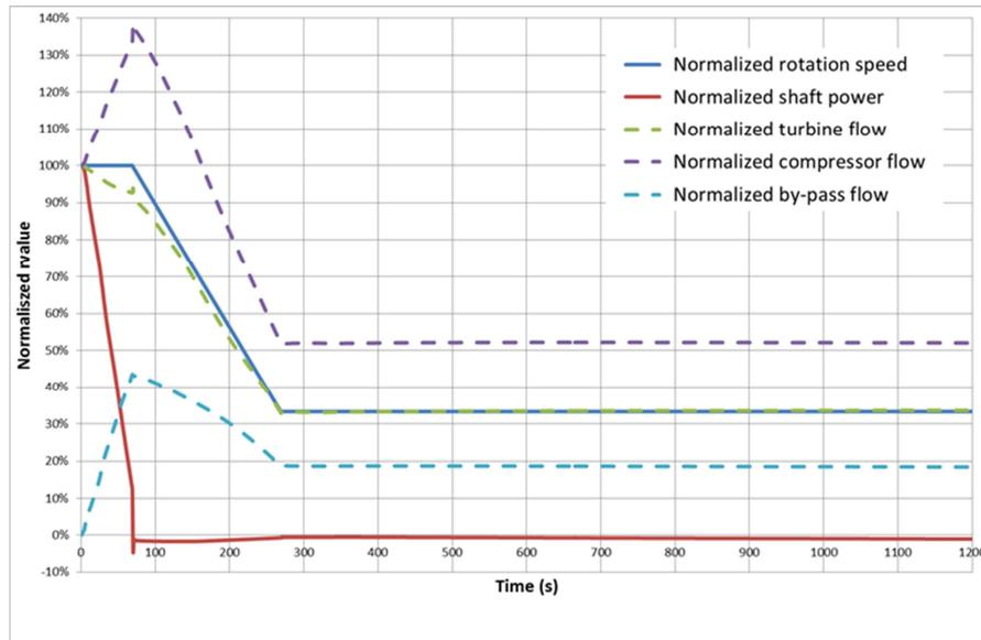
FIG.6: Evolution of the shaft speed and flowrate(normalized by its nominal value) during a SCRAM.
