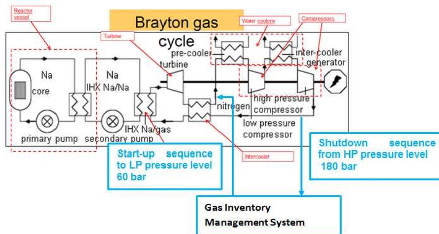
FIG 4: Scheme of gas inventory management system
