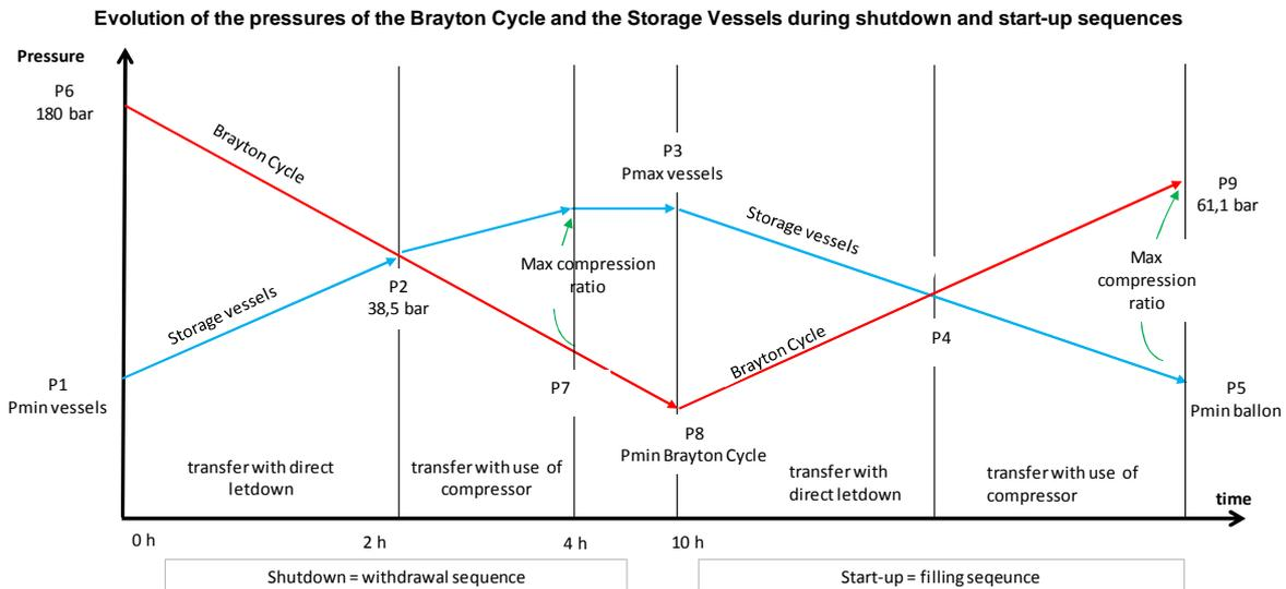
FIG 5 : Evolution of the pressures of the cycle and the storage vessels during shutdown and start-up sequences
