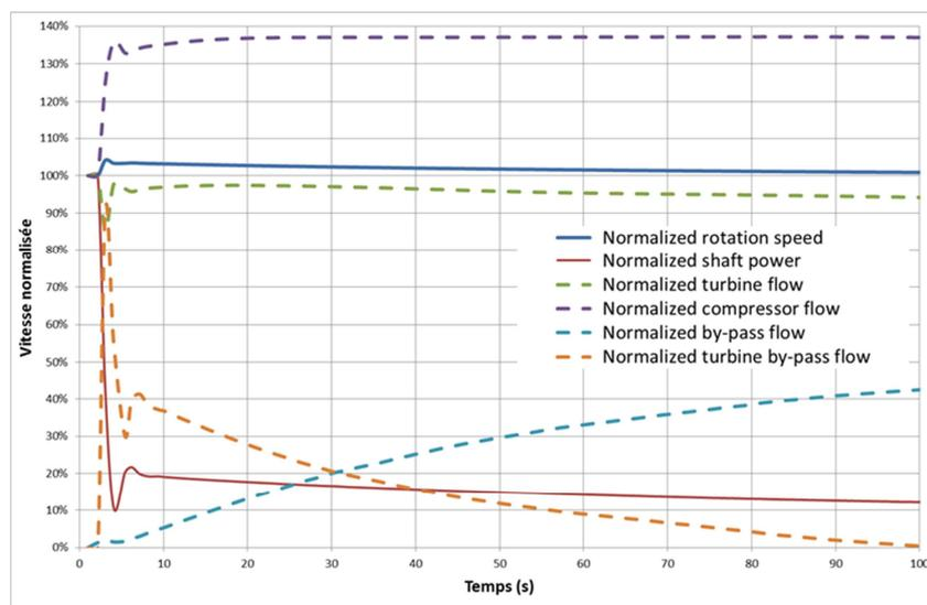
FIG 8: Shaft speed and gas flowrate (normalized by its nominal value) during a house load procedure.
