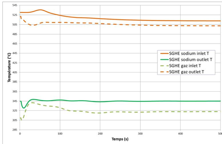
FIG. 9: Evolution of inlet and outlet temperature of the ECSG during a house load operation.
