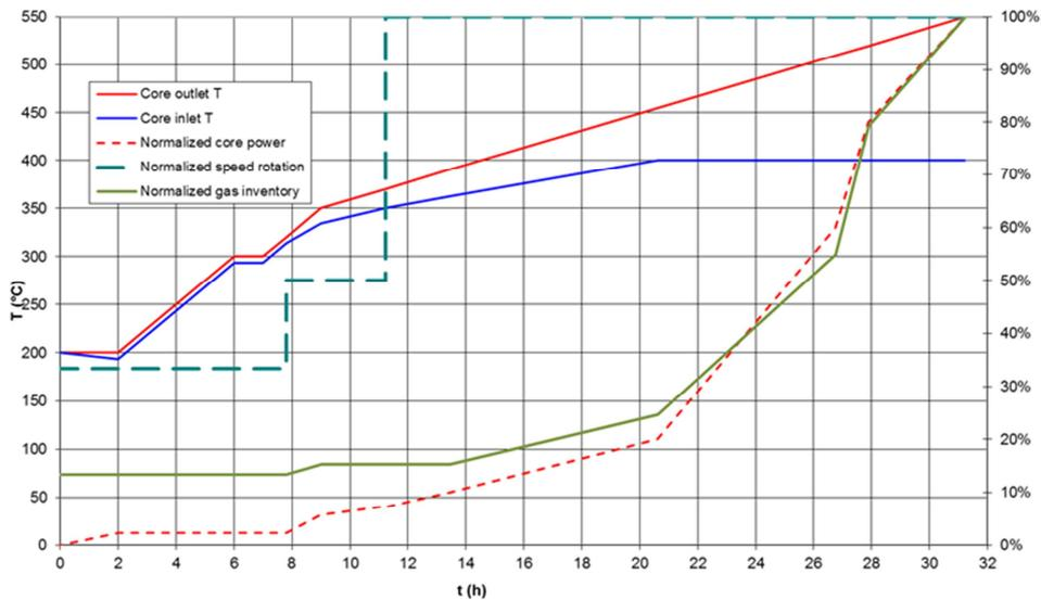
FIG 3: Operating parameters evolution during a normal shutdown
