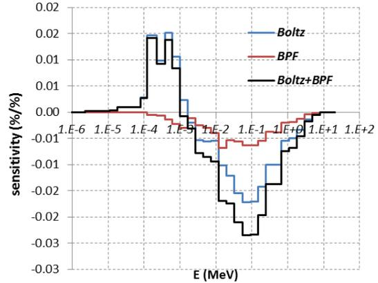
Fig. 6. Core Doppler sensitivity profile relative to Pu<sup>241</sup> fission cross section.
