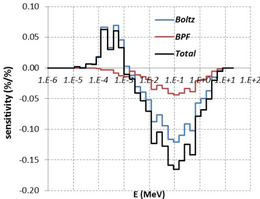
Fig. 5. Core Doppler sensitivity profile relative to Pu<sup>239</sup> fission cross section.
