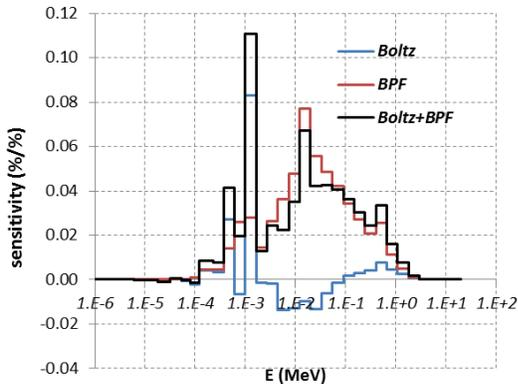
Fig. 4. Core Doppler sensitivity profile relative to U<sup>238</sup> capture cross.
