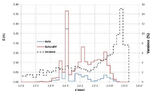
Fig. 10. Doppler U<sup>238</sup>(n,γ) uncertainty profile with incident neutron energy assuming no correlation using coupled and Boltzman sensitivities.
