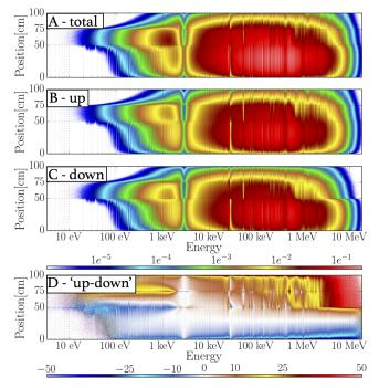
Fig. 10. Neutron flux normalized per source neutron: the "A" map represents the total flux, the "B" and "C" maps represent the neutrons with respectively a positive (up) and a negative (down) axial velocity, and the difference of "B-C" is presented in map "D" in percents of the average values.
