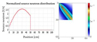
Fig. 2. Source neutron distribution (left) and reference  $G_{\chi_p \nu_p}$  matrix (right).
