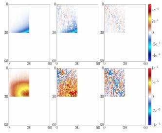
Fig. 4. Fission matrix variation due to a local variation of the sodium density of -2% in the sodium plenum (top) and to a local variation of the temperature of -300K (bottom): results of the interpolation model (left), direct Monte Carlo calculation (middle) and difference (right).
