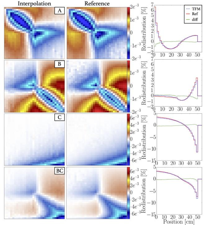
Fig. 8. TFM interpolated matrix variation (bins 0-30) associated to the -100 % sodium variation (left), reference matrix variation (middle) and comparison of the associated source neutron redistributions.
