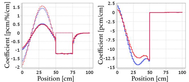
Fig. 9. Density feedback coefficient (left) associated to a local perturbation of -1 % in the sodium (plain line) and the steel (dashed line), and Doppler logarithmic coefficient (right) calculated as  $\frac{\Delta\rho}{\log(T+300/T)}$ , with TFM (red) and ERANOS (blue).
