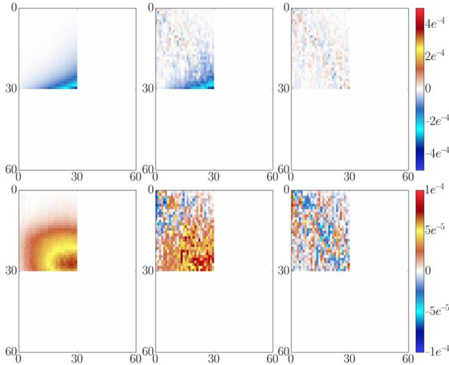
Fig. 4. Fission matrix variation due to a local variation of the sodium density of  $-2\%$  in the sodium plenum (top) and to a local variation of the temperature of  $-300\text{K}$  (bottom): results of the interpolation model (left), direct Monte Carlo calculation (middle) and difference (right).
