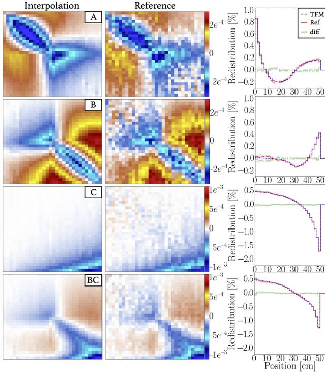
Fig. 7. TFM interpolated matrix variation (bins 0-30) associated to the -15 % sodium variation (left), reference matrix variation (middle) and comparison of the associated source neutron redistributions.
