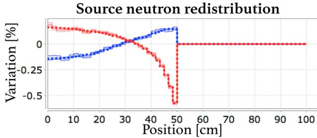
Fig. 5. Source neutron redistribution due to a local variation of the sodium density (red) and of the temperature (blue): results of the interpolation model (dashed line) and of the direct Monte Carlo calculation together with the statistical error (solid line).
