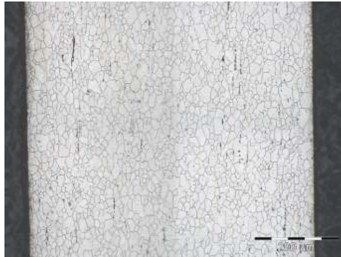
FIG. 1. Metallography of the cladding showing austenitic grains and primary carbide precipitates.
