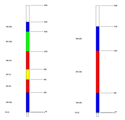
FIG. 6.Axial structure of the inner and outer fuel tubes  $Red = fuel - Blue = depleted UO_2 - Yellow = fertile plate - Green = Na$
