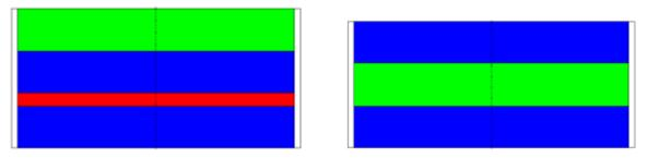
FIG. 4. Basic patterns (cells) of the pellet stacks for the fuel (left) and fertile plate (right) zones  $Red = Pu (metal) - Blue = depleted UO_2 - Green = Na$
