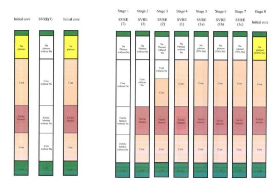
FIG. 7.Schematic view of the sodium voiding and filling sequences (white = voided) Note the progressive filling of the plenum:  $100\% \rightarrow 75\% \rightarrow 50\% \rightarrow 25\% \rightarrow 0\%$  void
