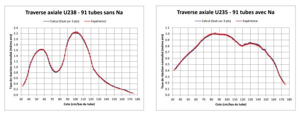
FIG. 9.Examples of axial traverses – Left:  $^{238}U(n,f)$  in the core with the 91 central tubes voided – Right:  $^{235}U(n,f)$  in the reference core. Blue = calculation (TRIPOLI-4+JEFF-3.1.1), Red = experiment Left ( $^{238}U$ ): bumps in the lower and upper fuel regions, depression in the fertile plate – Right ( $^{235}U$ ): smooth behavior in the fuel + plate region, increase in the sodium plenum
