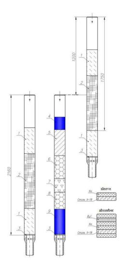
FIG. 8.Schematic view of a control rod mock-up tube fully inserted (left) and lifted (right) compared to a standard fuel tube (center)
