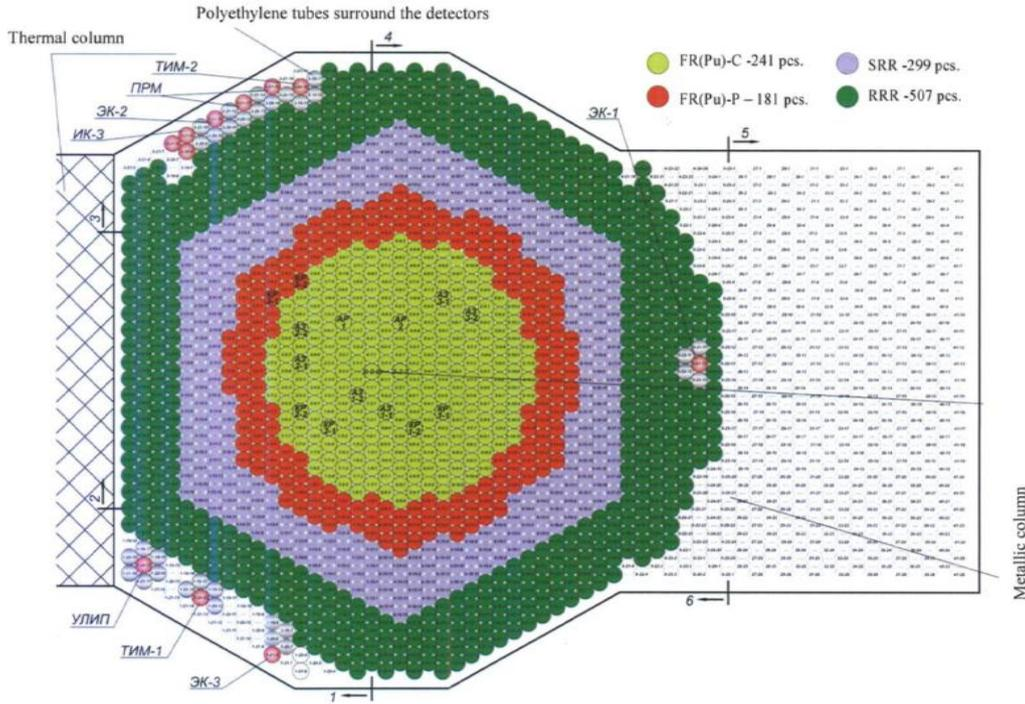
FIG. 5. Loading map of the BFS-115-1 reference core
