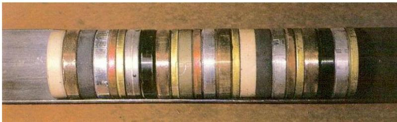
FIG. 3. Example of a pellet loading within a BFS tube (taken from [3])
