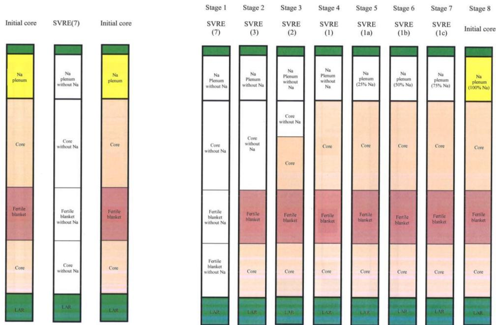
FIG. 7. Schematic view of the sodium voiding and filling sequences (white = voided)
