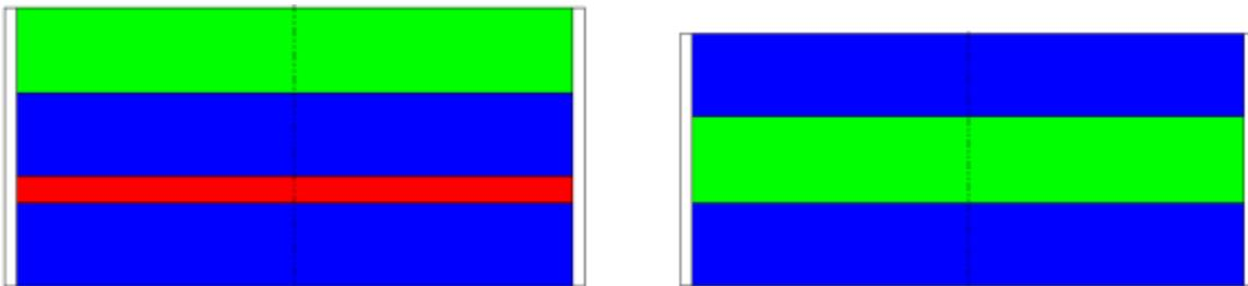
FIG. 4. Basic patterns (cells) of the pellet stacks for the fuel (left) and fertile plate (right) zones
