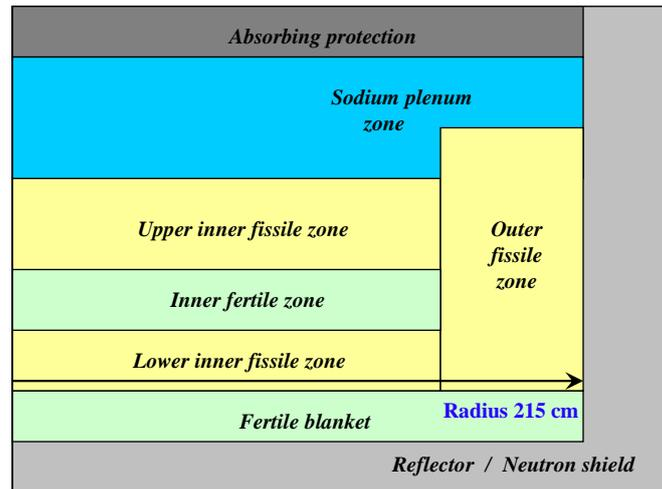
FIG. 1. Schematic R-Z cross-cut of the ASTRID core
