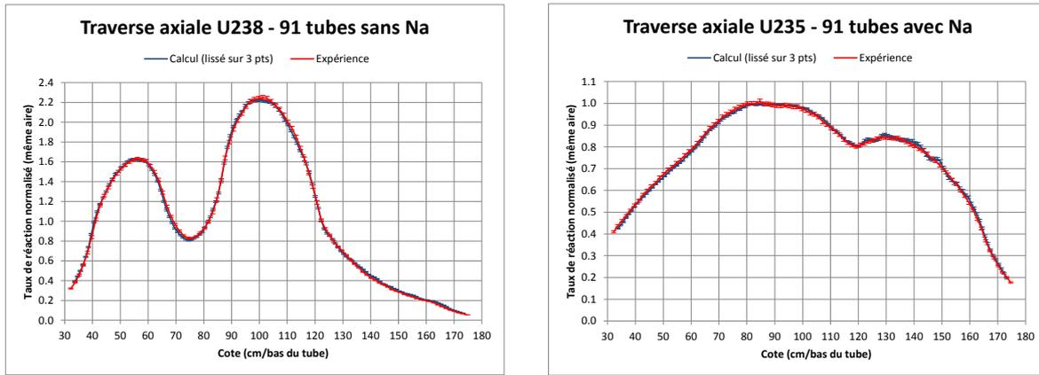
FIG. 9. Examples of axial traverses – Left:  $^{238}\text{U}(n,f)$  in the core with the 91 central tubes voided – Right:  $^{235}\text{U}(n,f)$  in the reference core. Blue = calculation (TRIPOLI-4+JEFF-3.1.1), Red = experiment
