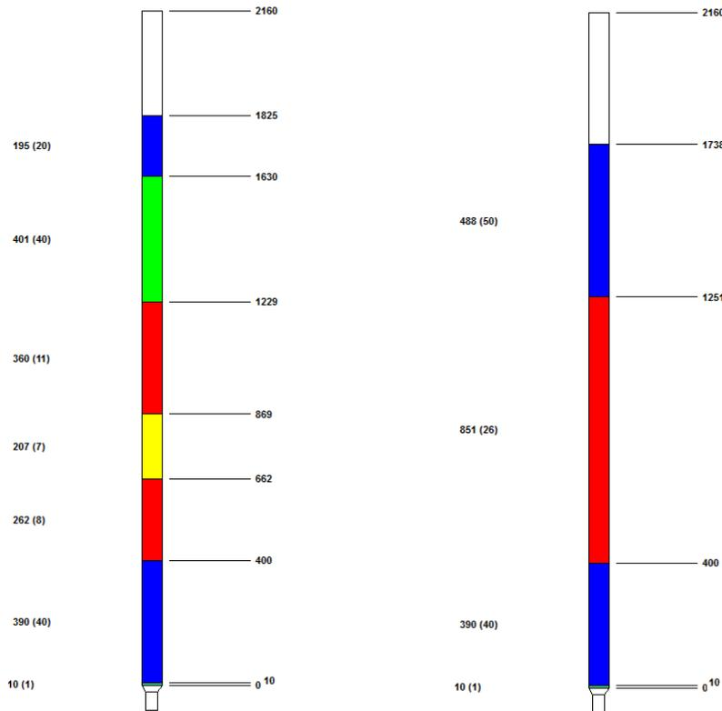
FIG. 6. Axial structure of the inner and outer fuel tubes
