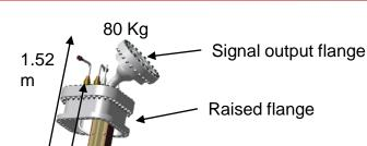
Small angle camera: 16 LOS, better resolution in plasma center and in lower divertor zone. Radial resolution of LOS at divertor 5 cm
