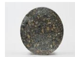
1 sample of **concrete** with L ~ 30 mm
