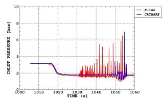
Figure 10: Inlet pressure during FC-34 test. Comparison between CATHARE-3 <u>rev3</u> calculations (in blue) and experiment (in red)
