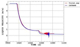
Figure 11: Inlet velocity during FC-21 test. Comparison between CATHARE-3 <u>rev3</u> calculations (in blue) and experiment (in red)
