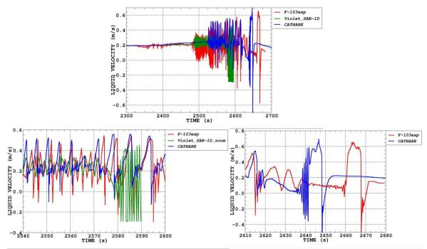
Figure 4: Inlet velocity during LHF-123 test. Comparison between CATHARE-3 <u>rev3</u> calculations (in blue), SABENA-1D calculations (in green) and experiment (in red)
