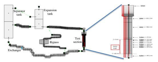
Figure 3: CATHARE modeling of SIENA loop and test section
