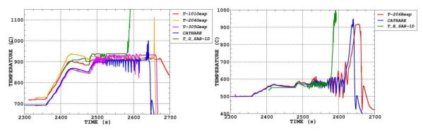
Figure 5: Pin temperatures during LHF-123 test at G plane (left) and B plane (right). Comparison between CATHARE-3 rev3 calculations (in blue), SABENA-1D calculations (in green) and experiment
