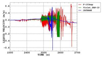
Figure 7: Inlet velocity during LHF-123 test. Comparison between CATHARE-3 <u>rev1</u> calculations (in blue), SABENA-1D calculations (in green) and experiment (in red)
