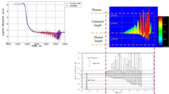
Figure 8: Inlet velocity (left) and void fraction map (right) during FC-34 test. Comparison between CATHARE-3 <u>rev3</u> calculations (in blue, top) and experiment (in red, bottom)
