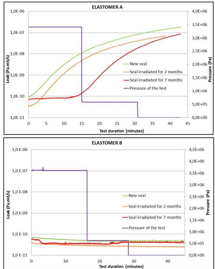
Fig. 3. Comparison of leak-tight behaviour between two different elastomers (fresh and after irradiation)
