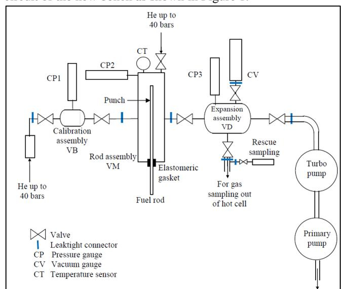
Fig. 1. Schematic diagram of the puncturing device
