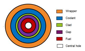
Figure 4. Axial cut of a subassembly (or a single pin in the CABRI channel).
