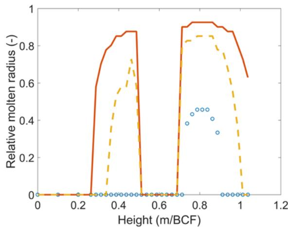
**Figure 13. Melting radius at the power peak (Solidus front E7 – solid, Liquidus front E7 – dotted, Solidus front E5 – circled, no liquidus front E5). The fuel is in a double-phase state between the solidus and the liquidus front.**
