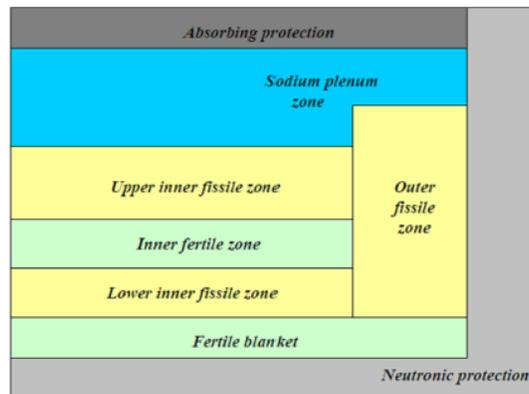
Figure 1. Radial cut of CFV core geometry.
