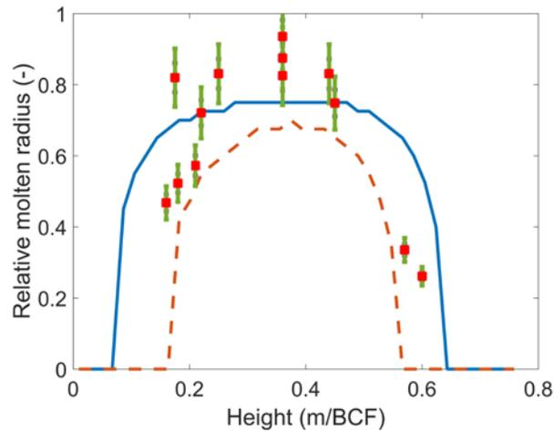
**Figure 6. Molten radius for E5 transients (Solidus front – solid, Liquidus front – dotted, Experimental double-phase front – squared). The fuel is in a double-phase state between the solidus and the liquidus front.**
