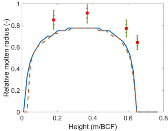
**Figure 8. Molten radius for E9 transients (Solidus front – solid, Liquidus front – dotted, Experimental double-phase front – squared). The fuel is in a double-phase state between the solidus and the liquidus front.**
