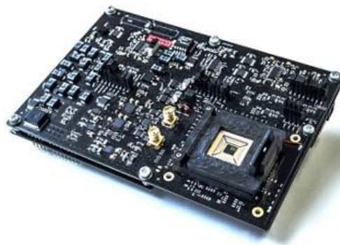
Figure 6: Photography of CreaPYX test system platform
