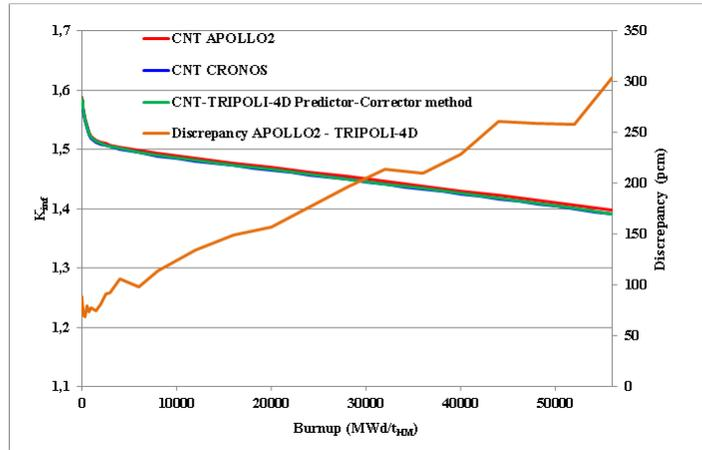
**Figure 10.**  $k_{inf}$  calculations for the CNT assembly – comparison between APOLLO2, CRONOS2 and TRIPOLI-4<sup>®</sup>D
