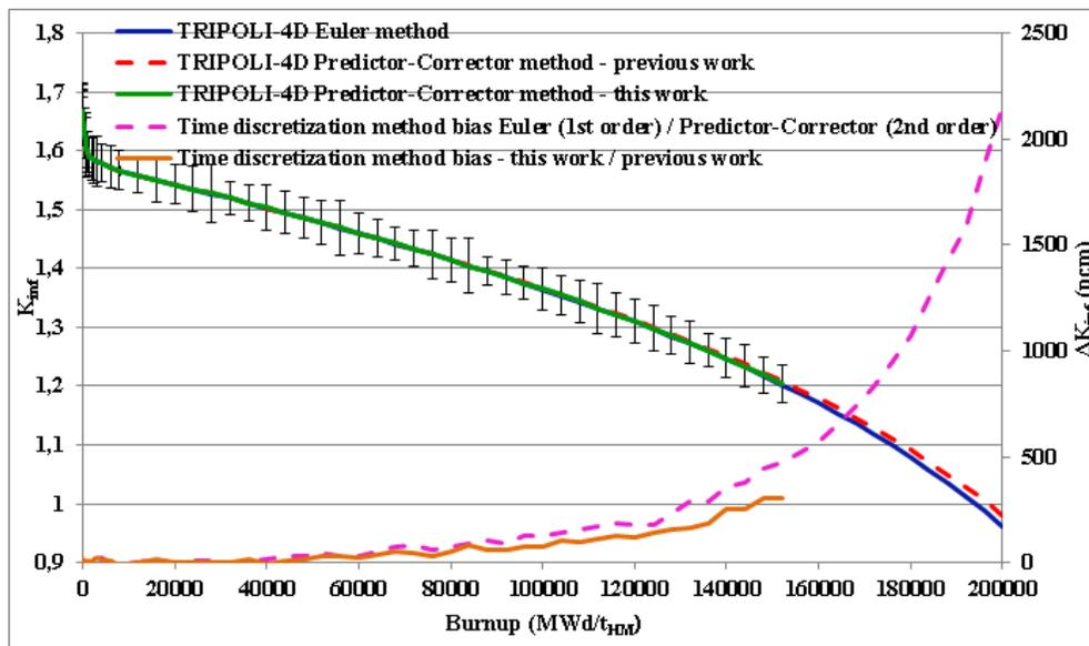
**Figure 5.** Evolution of the infinite multiplication factor in depletion and evaluation of the bias due to the time discretization methods: Euler (1<sup>st</sup> order) and Predictor-Corrector (2<sup>nd</sup> order) – STD assembly case
