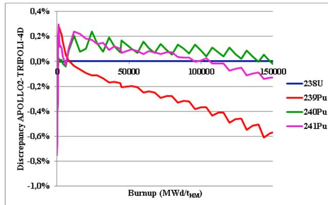
**Figure 8.** Evolution of the  $^{238}\text{U}$  chain isotopes masses in depletion: discrepancies APOLLO2-TRIPOLI-4<sup>®</sup>D – STD assembly case
