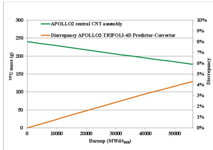
**Figure 11.** Evolution of the <sup>235</sup>U mass in depletion – comparison of APOLLO2 and TRIPOLI-4<sup>®</sup>D results in the CNT assembly case
