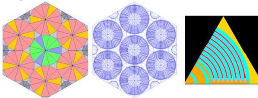
**Figure 4.** STD assembly with environment geometric pattern for CRONOS2 (left) and APOLLO2 (in the center) and TRIPOLI-4<sup>®</sup>D (right)
