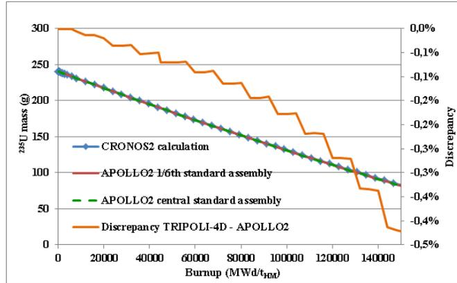
**Figure 7.** Evolution of the  $^{235}\text{U}$  mass in depletion – comparison of the APOLLO2, CRONOS2 and TRIPOLI-4<sup>®</sup>D results in the STD assembly case
