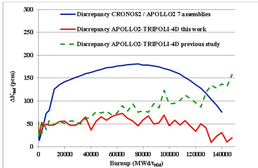
**Figure 6.**  $k_{inf}$  calculations for the STD assembly– comparison between APOLLO2, CRONOS2 and TRIPOLI-4<sup>®</sup>D
