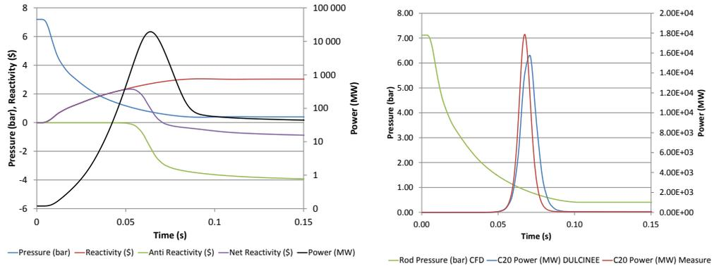
**Figure 9.** Computation with DULCINEE of a power transient using calculated gas pressure in transient rods. Case of a single depressurization from 7.2 *bar* (gas purity: 99.5%) through the high flow rate channel with the control valve fully opened (left)- Comparison of a computed power shape with measure for the C20 experiment (right)
