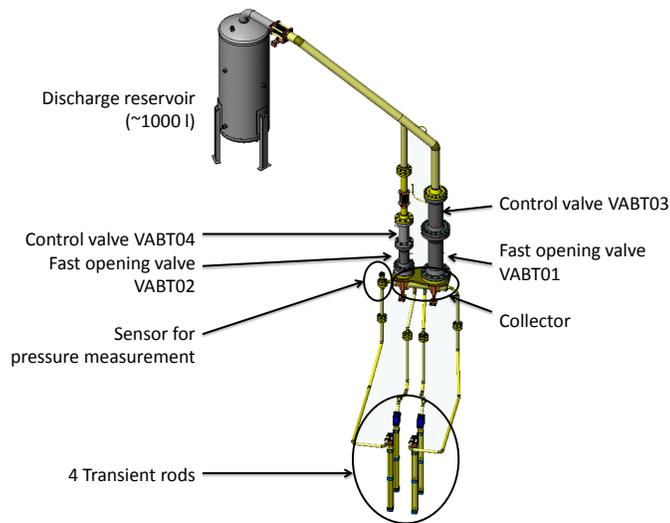
**Figure 2.** Main components of the CABRI transient rods
