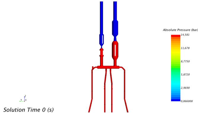
**Figure 4.** Pressure distribution before transient rods depressurization
