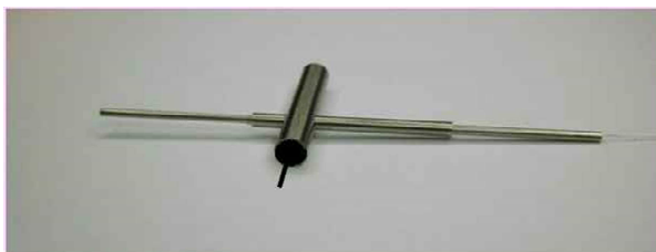
Fig. 8 : Optical module of the sensor inserted in a body with a piston simulating the feeler piece (CEA, R&D).
