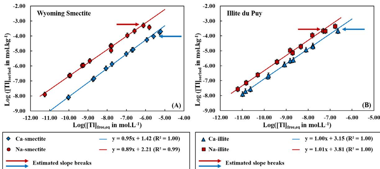
Fig. 2. Results in  $\log([Tl]_{\text{sorbed}}) = f([Tl]_{\text{free,eq}})$  for smectite (A) and illite (B). Error bars correspond to the variability of Tl sorbed. pH condition are  $7.34 \pm 0.40$ ,  $7.89 \pm 0.20$ ,  $5.00 \pm 0.10$  and  $7.18 \pm 0.08$  for respectively Na-smectite, Ca-smectite, Na-illite and Ca-illite (Figs. 3B, 4B, 5B and 6B captions).
