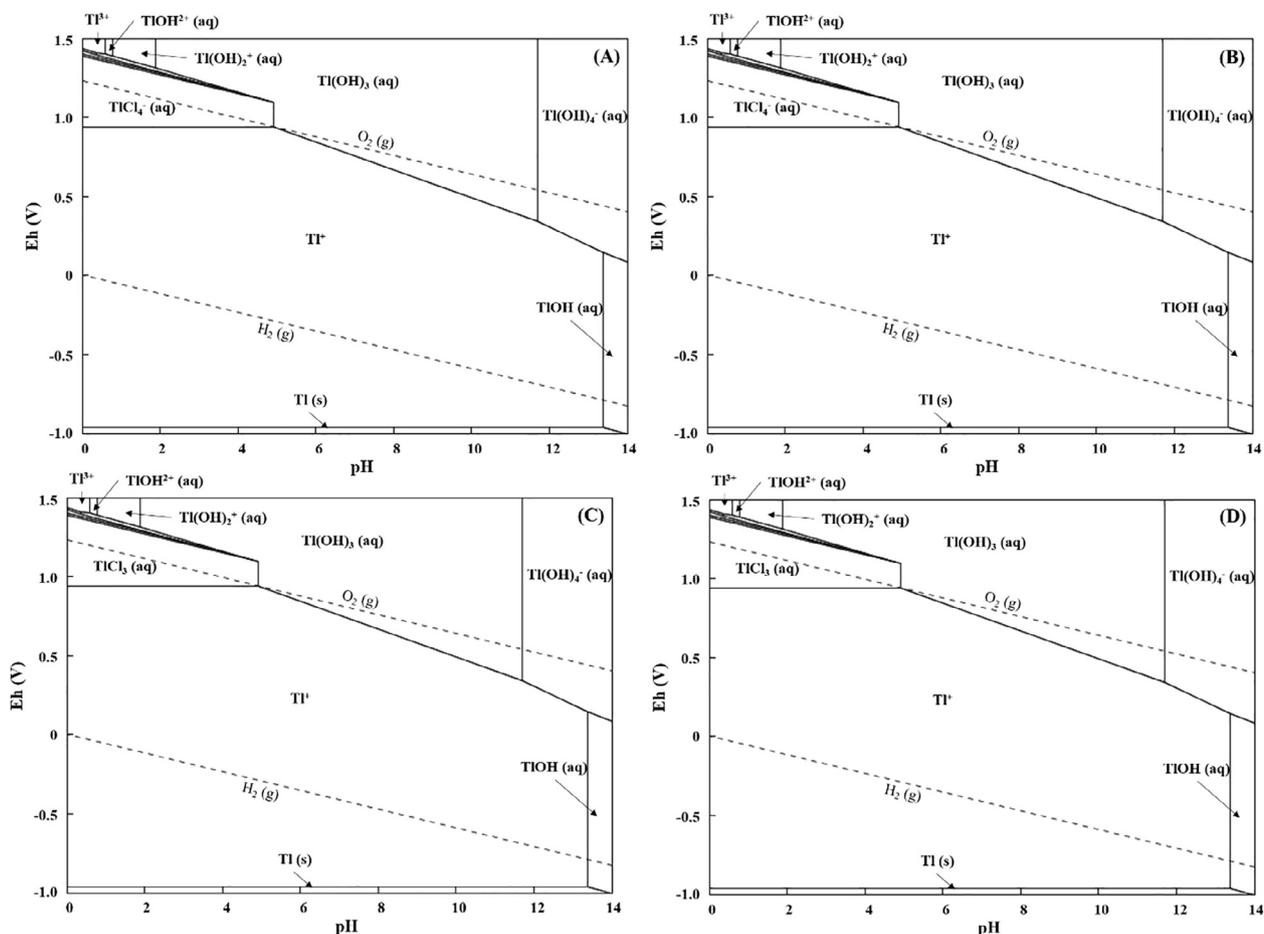
Fig. 1. Eh-pH diagrams for thallium. A Tl-Ca-Cl-H<sub>2</sub>O system is described for A and B with [CaCl<sub>2</sub>] = 10 mM. In A, [Tl] = 100 nM and in B, [Tl] = 0.1 nM. C and D describe a Tl-Na-Cl-H<sub>2</sub>O system with [NaCl] = 10 mM and [Tl] = 100 nM for C and 0.1 nM for D. Tl constants database is from Casiot et al. (2011) except for TlOH(aq) which is calculated from Brown and Ekberg's book (2016). Diagrams made with JChess v2.0.
