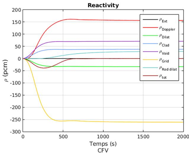
**Fig. 7.** Reactivity evolution of the CFV core during an ULOHS without minor actinides.
