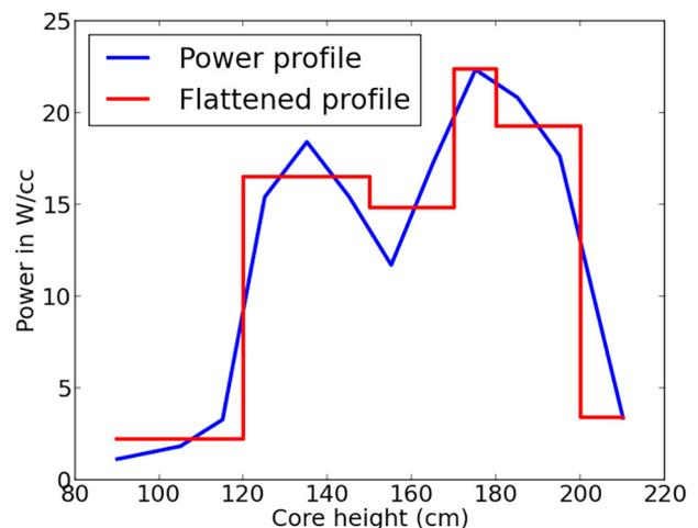
Fig. 3. Comparison of the real power profile and the flattened profile considered for this study.
