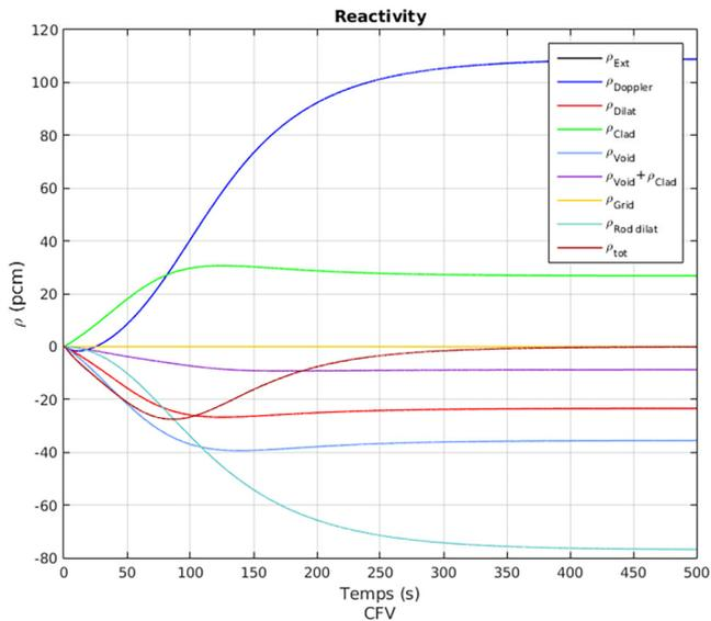
**Fig. 5.** Reactivity evolution of the CFV core during an ULOF without minor actinides.
