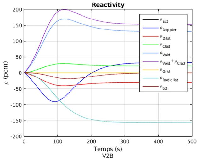
**Fig. 4.** Reactivity evolution of the V2B core during an ULOF without minor actinides.
