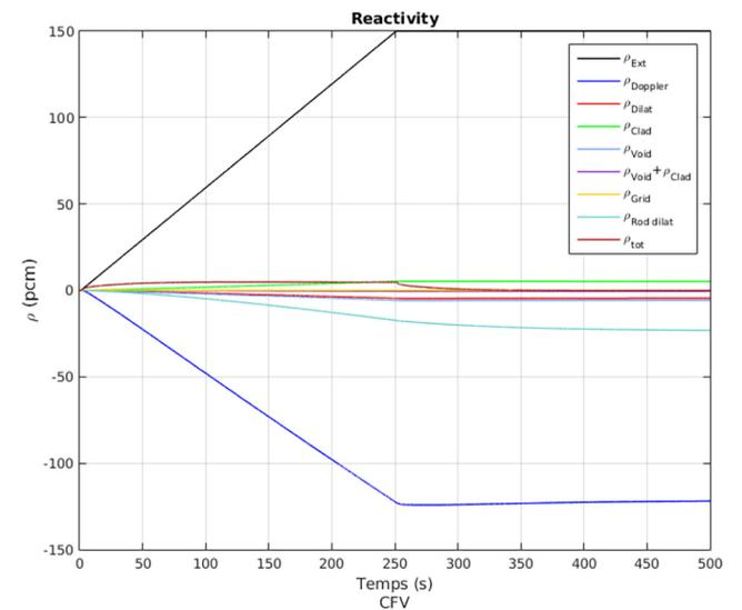
**Fig. 9.** Reactivity evolution of the CFV core during an UTOP without minor actinides.
