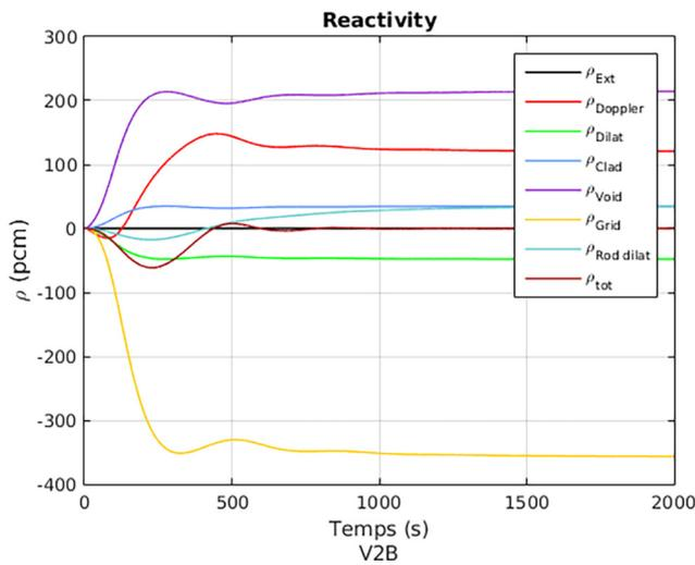
**Fig. 6.** Reactivity evolution of the V2B Core during an ULOHS without minor actinides.
