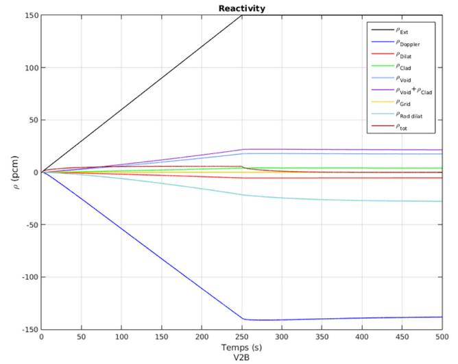
**Fig. 8.** Reactivity evolution of the V2B core during an UTOP without minor actinides.
