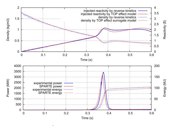
Fig. 11. Experimental/calculation comparison for <sup>3</sup>He density and core power including the TOP effect surrogate model.
