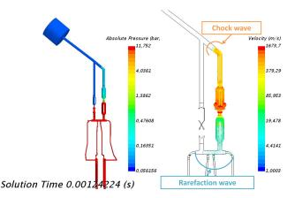
Fig. 2. Visualization of  ${}^{3}$ He transient rods depressurization with STAR-CCM+ – pressure (left) – velocity (right).
