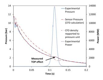
Fig. 7. CFD calculation of simple depressurization by high flow rate channel (VABT03 aperture  $\sim$ 40%) including TOP effect.
