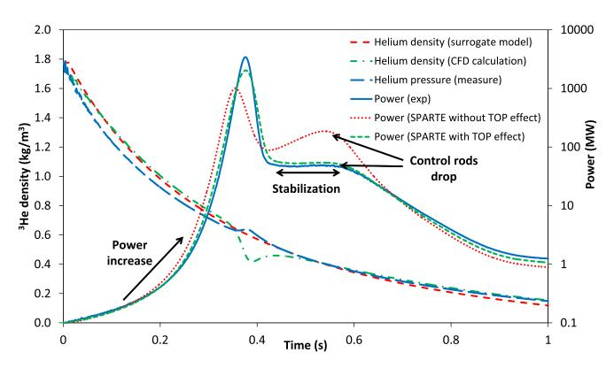
Fig. 10. Comparison of measured CABRI power transient and power transients calculated with density surrogate model and CFD calculation including TOP effect—case of low flow rate channel depressurization.
