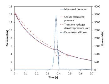
Fig. 9. CFD calculation of simple depressurization by low flow rate channel (VABT04 aperture  $\sim$ 30%) including TOP effect.
