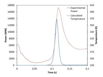
Fig. 8. Evolution of  ${}^{3}$ He temperature in transient rods according to CFD calculation.
