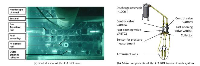
Fig. 1. CABRI transient rod system. (a) Radial view of the CABRI core. (b) Main components of the CABRI transient rod system.
