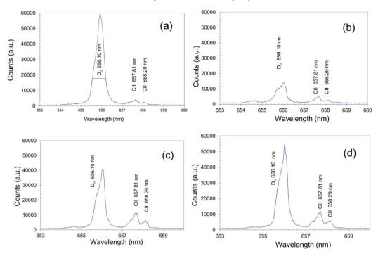
**Fig. 5.** LIBS spectrum of deuterium and carbon in zone 2 after the 1st (a), 2nd (b), 3rd (c) and 4th (d) laser shot on the W-stripe zone with the DL (200  $\mu$ m spectrometer slit width, 1800 mm<sup>-1</sup> grating, 180 ns ICCD camera delay, 10  $\mu$ s gate width, MCP gain = 100, vacuum). Laser pulse energy E = 2.9 J (a), 3.0 J (b), 3.5 J (c) and 3.8 J (d). Spectral line asymmetry is related with the spectrometer particular feature on the spectral range of 630–660 nm.
