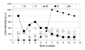
**Fig. 4.** In-depth characterisation of the DL (zone 1).  $D_{\gamma}$  WI, Bell, CII and CrI spectral line intensities are presented as a function of a number of applied laser shots.
