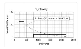
**Fig. 7.**  $D_{\alpha}$  spectral line (656 nm) decrease with the time delay (solid line rectangulars). An approximation of  $D_{\alpha}$  spectral line exponential decrease for the time delay derives  $\tau \approx 700$  ns (a dashed line).
