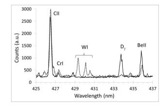
**Fig. 3.** LIBS spectrum after the 1st (solid curve) and 10th laser shot (pointed curve) on the W-stripe zone with the DL in zone 1 (laser pulse energy  $E = 3.2 \pm 0.5$  J, 200 µm spectrometer slit width, 1800 mm<sup>-1</sup> grating, 180 ns ICCD camera delay, 10 µs gate width, MCP gain = 25, vacuum).
