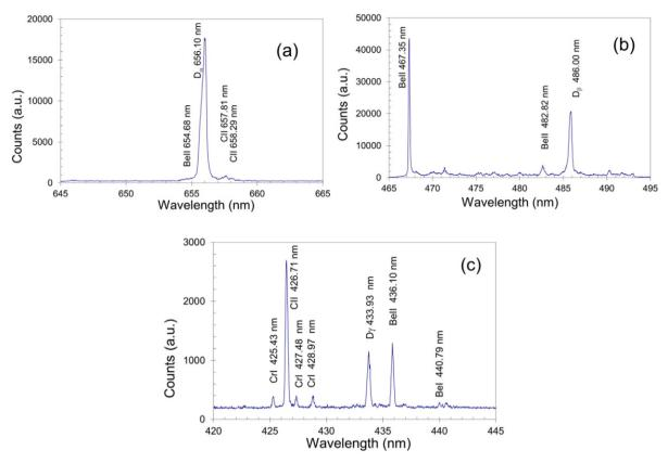
**Fig. 2.** The examples of LIBS spectra obtained from DL on the JET divertor tile with the laser pulse energy ( $E = 3.2 \pm 0.5$  J) and with the optimal set of registration parameters: 200 µm spectrometer slit width, 180 ns ICCD camera delay, 10 µs gate width, vacuum. (a) E = 3.0 J, MCP gain = 25, after 1st laser shot, (b) E = 3.3 J, MCP gain = 100, after 5th laser shot, (c) E = 3.0 J, MCP gain = 100, after 1st laser shot.
