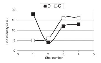
Fig. 6. In-depth characterisation of the DL for zone 2.  $D_{\alpha}$  and CII spectral line intensities are presented as a function of a number of applied laser shots.
