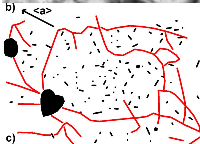
Figure 2 : a) Imaging of nano-precipitates and dislocation with a diffraction vector g=11\bar{2}0 and the electron beam close to the zone axis B\sim[0002] . The corresponding diffraction pattern is shown encapsulated. b) a zoom on the center of the picture is also shown. c) Detailed drawing showing the dislocations and beta-Nb nano-precipitates.
