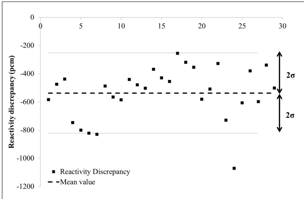
**Fig.10. Scheme bias and uncertainty on reactivity calculation for rodged core configurations at step 0**
