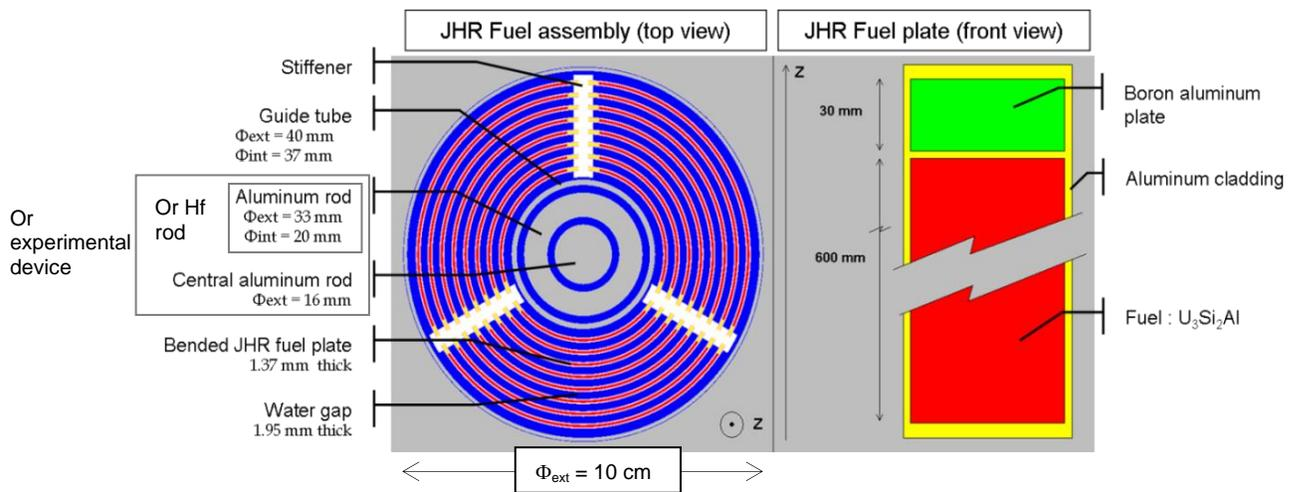
**Fig.2. JHR fuel element and JHR fuel plate description**
