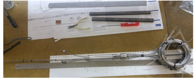
Fig. 12. Thermocouples (bottom part of the picture) ready to be assembled in the TZM shroud (top part of the picture).
