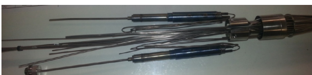
Fig. 11. The two pressure transducers and the thermocouples.
