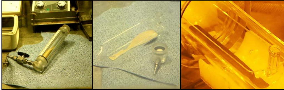
Figure 1 : Pictures of U-Am oxide microspheres synthesis in hot cell in Atalante facility. From left to right: loaded resin in plexiglass column, loaded resin in the quartz crucible before calcination in airflow and oxidized (U,Am)_3O_8 microspheres.
