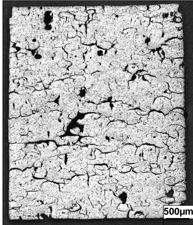
Figure 5 : Optical microscopic observation of the internal microstructure of sintered (U,Am)O<sub>2</sub> porous pellet.
