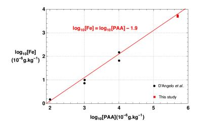
**Figure 4 :** Evolution of the iron concentration logarithm as a function of the PAA concentration logarithm after interaction at 275 °C with 20 min residence time. The black points are from the study of D'Angelo *et al.* [6] and the red squares are from this study
