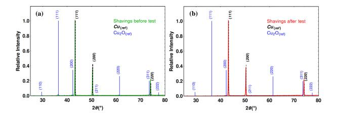
Figure 2 : (a) X-ray diffraction pattern of copper shavings before interaction with PAA, JCPDS data for metallic copper (Cu<sub>(ref)</sub>) and for copper oxide (Cu<sub>2</sub>O<sub>(ref)</sub>) (b) X-ray diffraction pattern of copper shavings after interaction with PAA at 275 °C with a 20 min residence time
