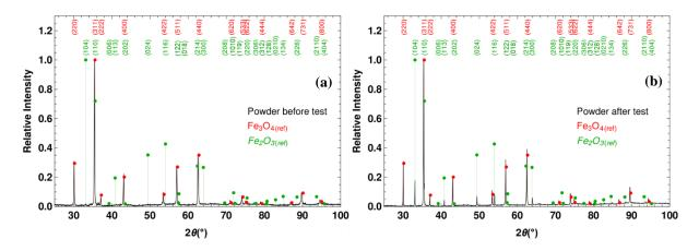
Figure 3 : (a) X-ray diffraction pattern of the tested magnetite powder before interaction with PAA, JCPDS data for magnetite (Fe<sub>3</sub>O<sub>4</sub> in red) and for hematite (Fe<sub>2</sub>O<sub>3</sub> in green) (b) X-ray diffraction pattern of the tested magnetite powder after interaction with PAA at 275 °C with a 20 min residence time
