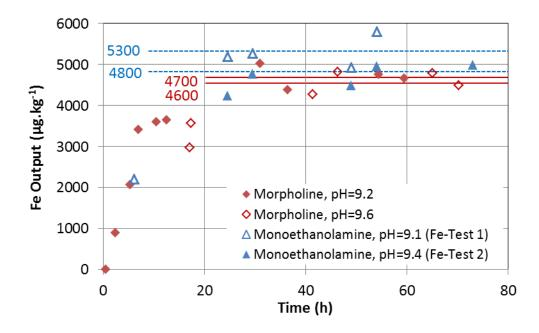
**Figure 6:** Evolution of iron content in the solution for the monoethanolamine and morpholine chemical conditionings. The samples were realized at the output of the device for a residence time equal to 20 min.
