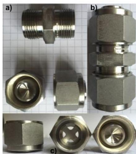
**Figure 1.** Open Swagelok connector (a), closed experimental capsule (b), stainless steel separator (c).
