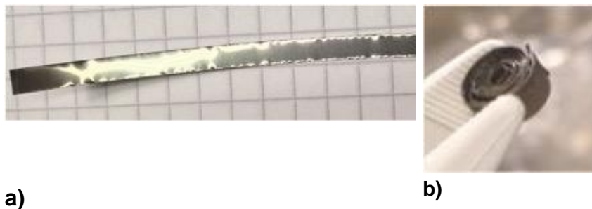
Figure 7. Niobium metal strip used as oxygen buffer before (a) and after the reaction (b)
