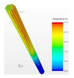
Fig. 6. Cladding temperature distribution of MgO-pins bundle – Without sodium flow.
