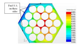
Fig. 7. Sodium temperature distribution in S/A in core mid-plane – Without sodium flow.
