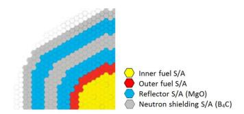
Fig. 4. Radial shielding of ASTRID core CFV v3.
