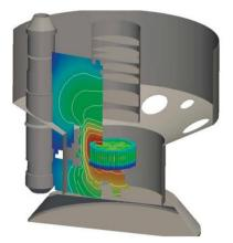
Fig. 3. MCNP calculation of neutrons streaming from core to IHX.
