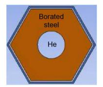
Fig. 10. Design of borated steel shielding S/A (section view).
