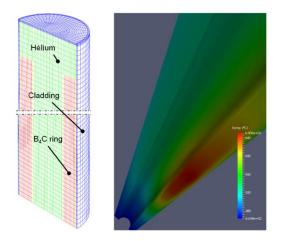
Fig. 9. Thermomechanical simulation on B<sub>4</sub>C sealed cylinder. Temperatures (°C) in B<sub>4</sub>C rings.
