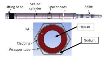
Fig. 8. Basic design of B<sub>4</sub>C radial shielding S/A. Side view (top) and section view (bottom).
