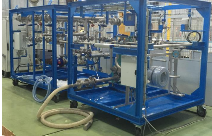
Figure 5 : Mock-up facility for Hydraulic Tests
