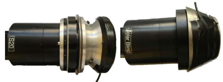
View of tubes equipped with ALADIN pinhole and 25 mm diameter scintillator
