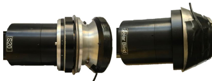
View of tubes equipped with ALADIN pinhole and 25 mm diameter scintillator
