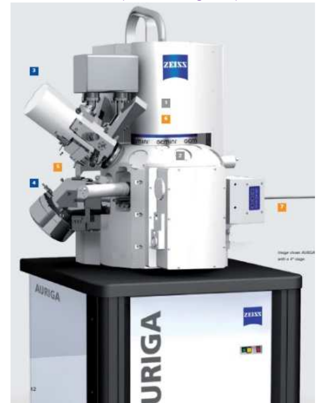
Non nuclearized FIB-SEM (Zeiss Auriga 40)
